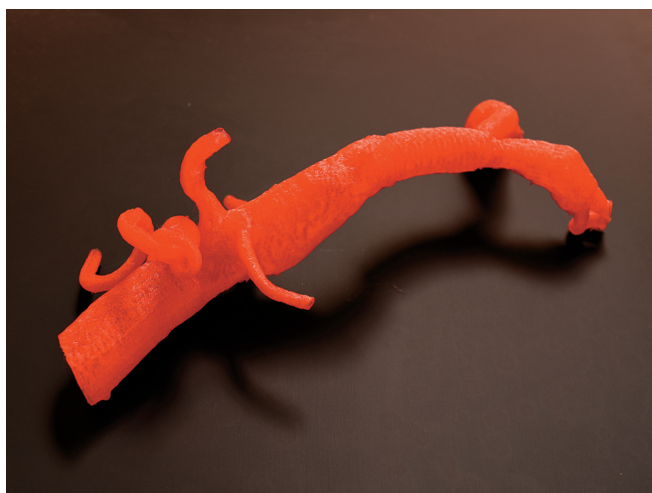
Figure 3.—3D printed abdominal aorta.
